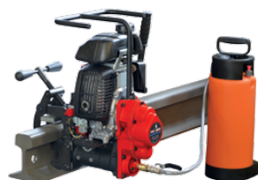
PRO-36 RH • Core drill: max 36 mm • Petrol motor
