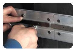
The tool removes the gap between gear racks
