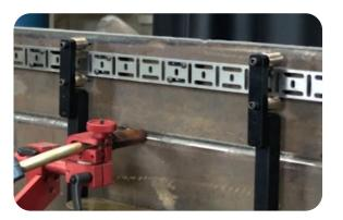
Guide adjustment tool to position the track parallel to the edge
